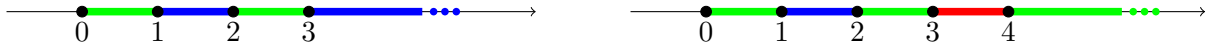
Figure 2 The partition on the right is a laminar partition corresponding to the laminar interval family \mathcal{I}_1 = [0, \infty) , \mathcal{I}_2 = [1, 2) and \mathcal{I}_3 = [3, 4) , while the partition on the left is not a laminar partition.
