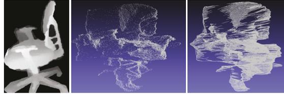
Figure 2. An example depth map of a chair (left), the reconstructed point cloud (middle), and the mesh model (right).
