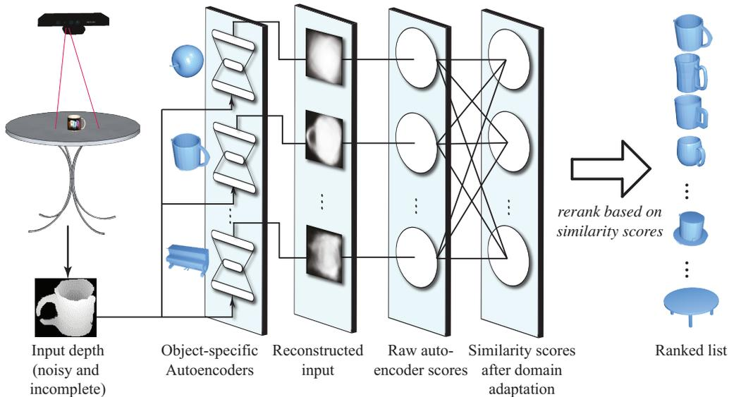
Figure 3. The architecture of our retrieval system, from a neural network perspective. The 3D model next to each autoencoder indicates the CAD model from which the autoencoder is trained.
