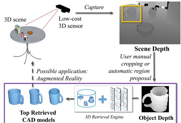
Figure 1. 3D shape retrieval using one depth image from a low-cost sensor. The purple rectangle shows the scope of this paper.
