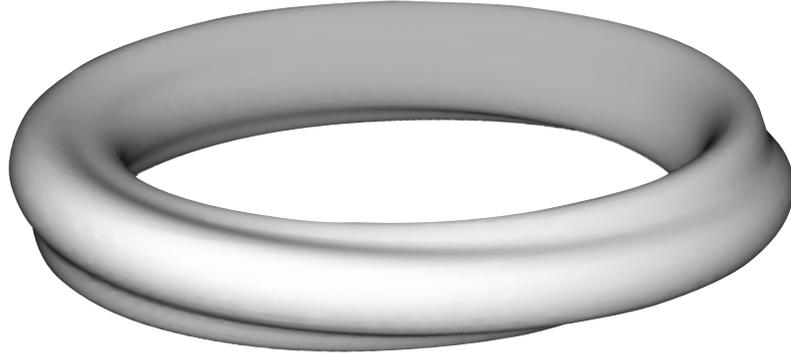
**Fig. 2.3:** An  $(m, n) = (3, 1)$  perturbation to a toroidal surface, such as might be observed during the onset of an external kink mode.
