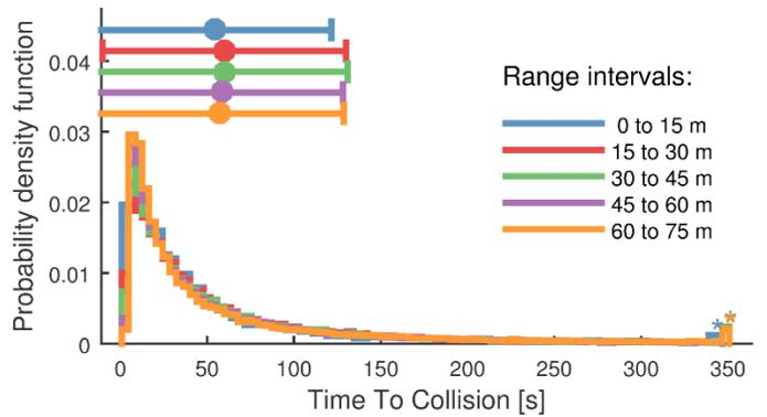
Fig. 8. Distribution of  $TTC_L(t_{LC})$  with variant  $R_L(t_{LC})$  intervals
