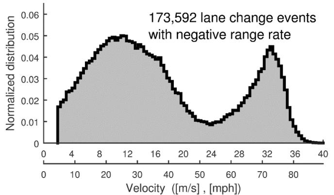
Fig. 3. Distributions of  $v_L(t_{LC})$  of the lane change events used the our model
