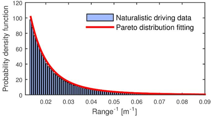
Fig. 5. Fitting results of  $R_L^{-1}(t_{LC})$  using the Pareto distribution
