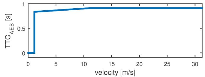
Fig. 9.  $TTC_{AEB}$  as a function of vehicle speed
