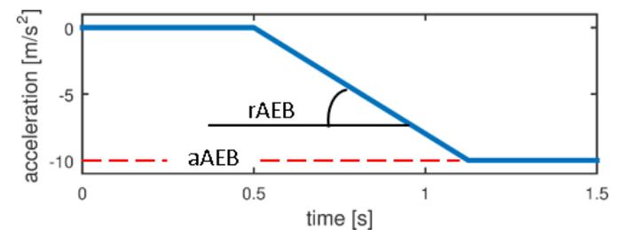
Fig. 10. The modeled AEB algorithm
