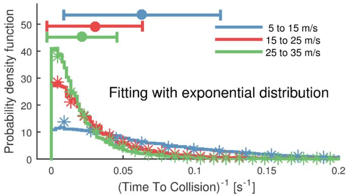
Fig. 6. Distribution of  $TTC_L^{-1}(t_{LC})$  at different lane change vehicle speeds
