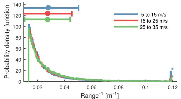
Fig. 4. Distributions of  $R_L^{-1}(t_{LC})$  at different vehicle forward speeds
