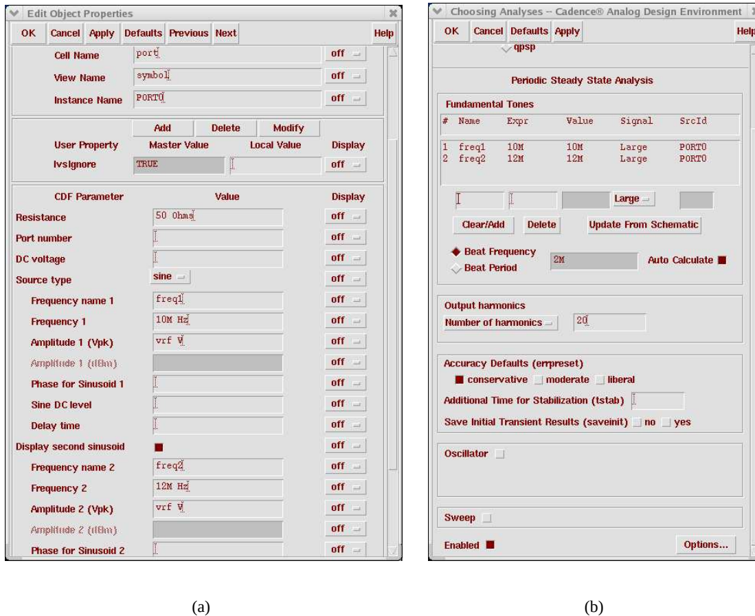
Fig. 4. (a) Properties of the port used in the test setup of fig. 3(a) (b) PSS analysis form.
