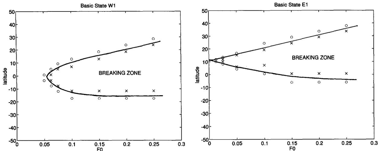
FIG. 12. Variation of surf zone width with forcing amplitude  $F_0$  for (a) basic state  $\mathcal{W}_1$ , and (b) basic state  $\mathcal{E}_1$ . A circle corresponds to a contour that remains single valued, and a cross to a contour that becomes double valued. The region between the curves (which have been drawn by hand) corresponds to the region of breaking (surf zone).
