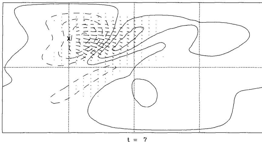
FIG. 10. Plot of wave activity flux vectors  $\mathbf{F}$ , and contours of perturbation streamfunction  $\psi^*$ , at day 7 for calculation W05 ( $F_0 = 0.05$  and basic state  $\mathcal{W}_1$ ). The contour interval of  $\psi^*$  is  $2.5 \times 10^6 \text{ m}^2 \text{ s}^{-1}$ .
