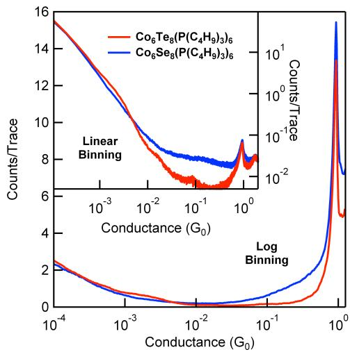
**Figure S-3.** Logarithmically binned conductance histograms for compounds **7** (in red) and **8** (in blue). Inset: Same histograms generated using linear bins.
