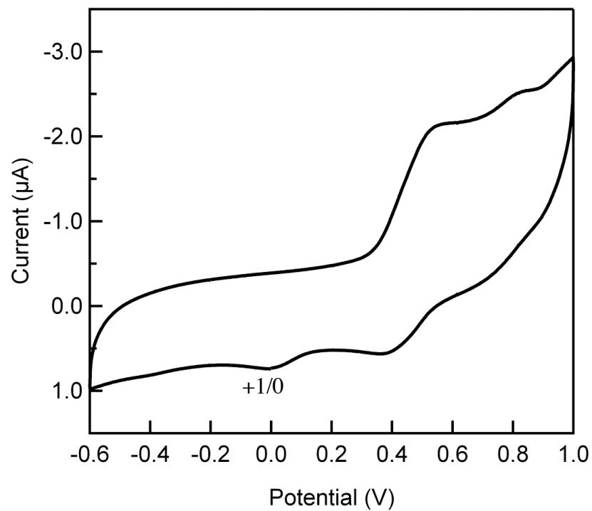
**Figure S-4.** CV trace of  $\text{Co}_6\text{Te}_8(\text{PEt}_3)_6^{+1}$  in 0.1 M TBAPF<sub>6</sub> in dichloromethane.
