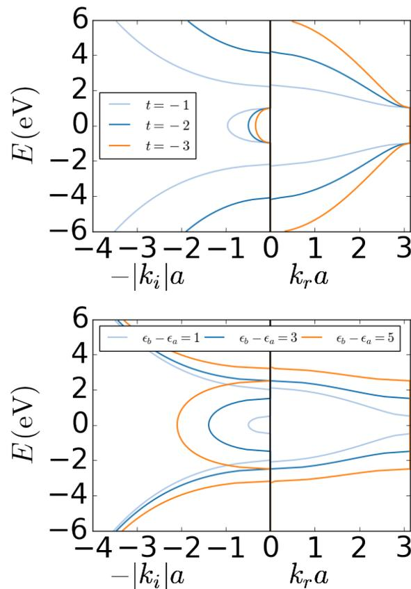
Figure S16. Complex band structure of an infinite chain of alternating sites. Top: the hopping element  $t$  is varied while the onsite energies are constant. Bottom:
