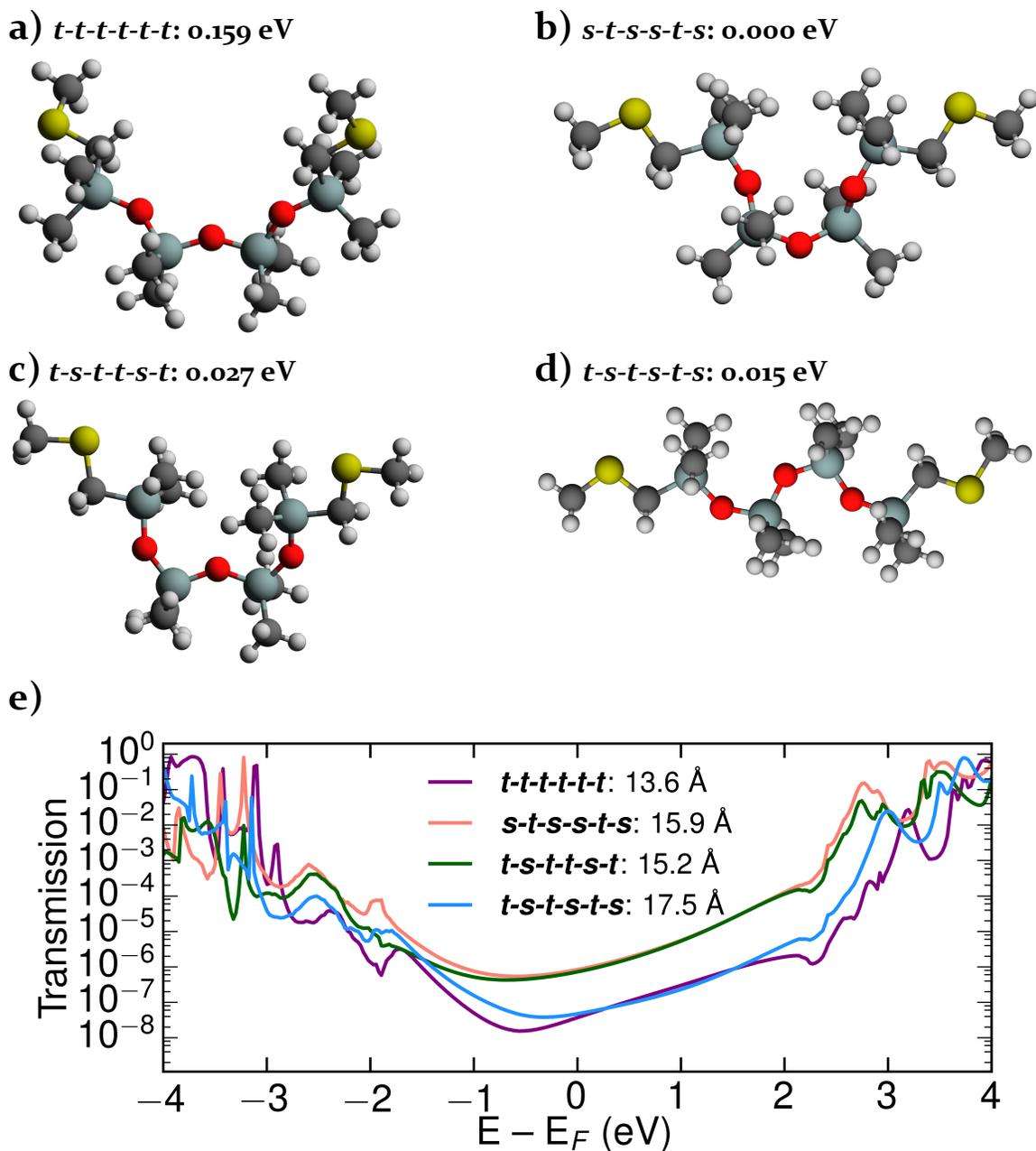
Figure S10. abcd) Optimized vacuum conformations of siloxane **3** and energy relative to the most stable conformation. e) transmission plotted semilogarithmically against energy. Junction tip-to-tip Au-Au length is listed.
