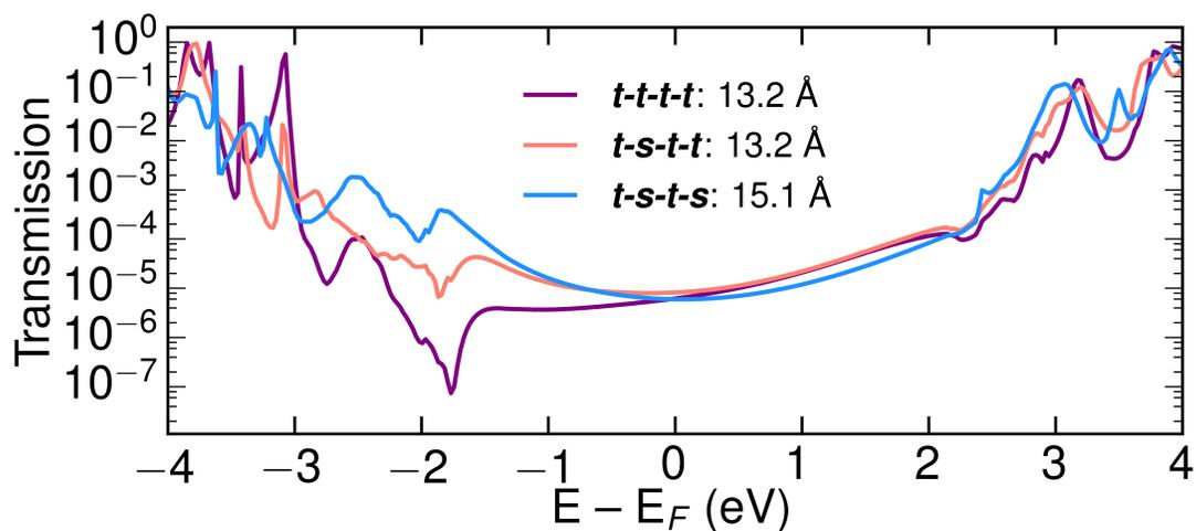
Figure S9. abc) Optimized vacuum conformations of siloxane **2** and energy relative to the most stable conformation. d) transmission plotted semilogarithmically against energy. Junction tip-to-tip Au-Au length is listed.
