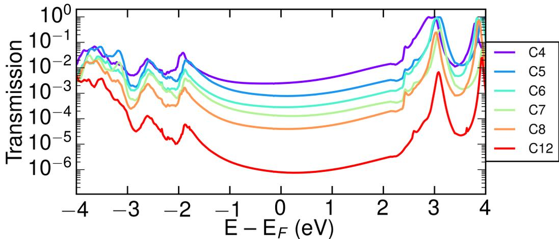
Figure S4. Transmission curves for linear alkanes C<sub>4</sub>-C<sub>8</sub> and C<sub>12</sub>.
