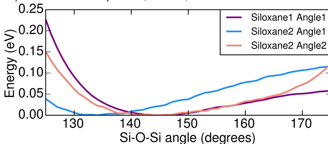
Figure S7. Total energy of siloxane 1 and siloxane 2 where the Si-O-Si bond angle is varied. The energy zero is set to that of the optimized structure.
