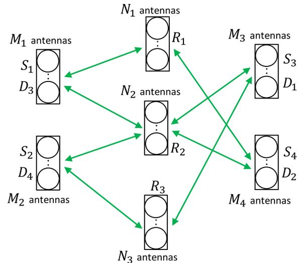
Fig. 1. A two-way MIMO butterfly interference network.
