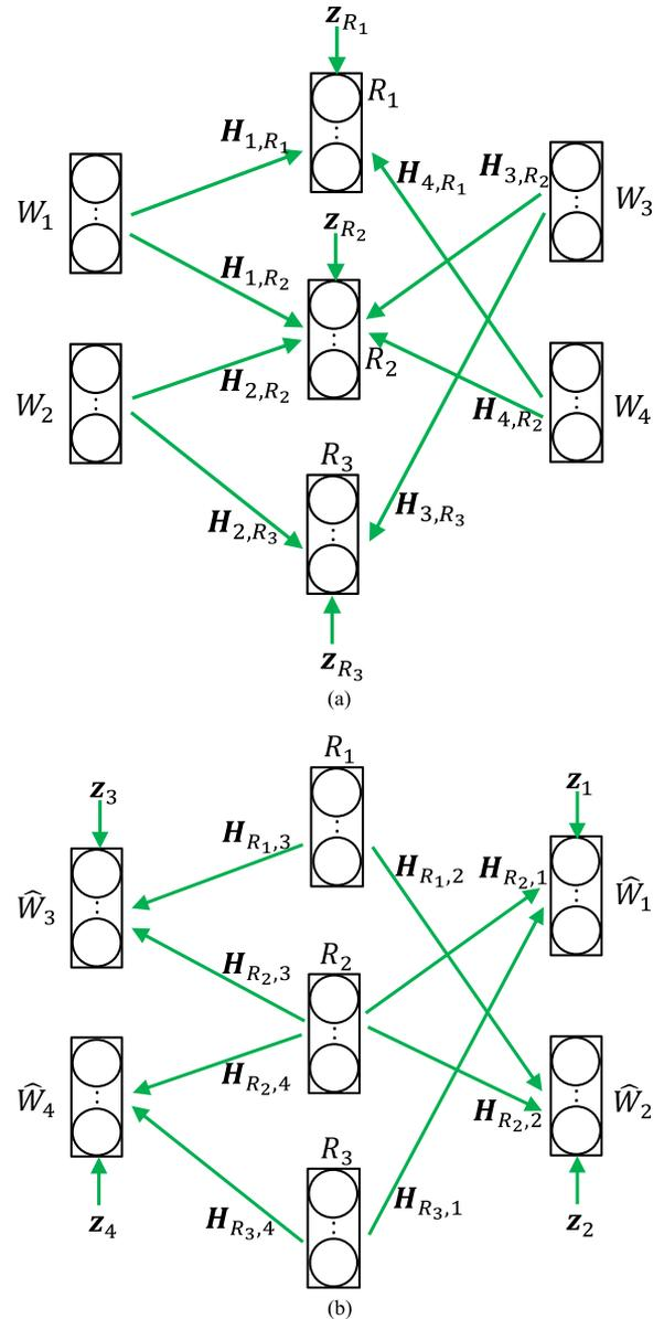
Fig. 2. The channels from and to relays in a two-way MIMO butterfly network. (a) The channels from transmitters to the relays. (b) The channels from relays to the receivers.
