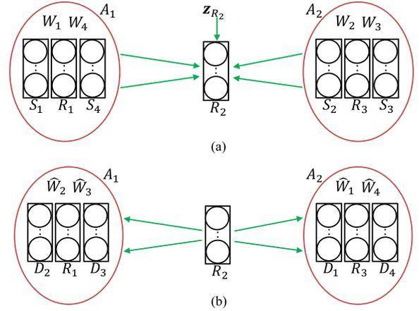
Fig. 3. The genie-aided MIMO butterfly network. (a) The channels from the transmitters to relay  $R_2$ . (b) The channels from relay  $R_2$  to the receivers.
