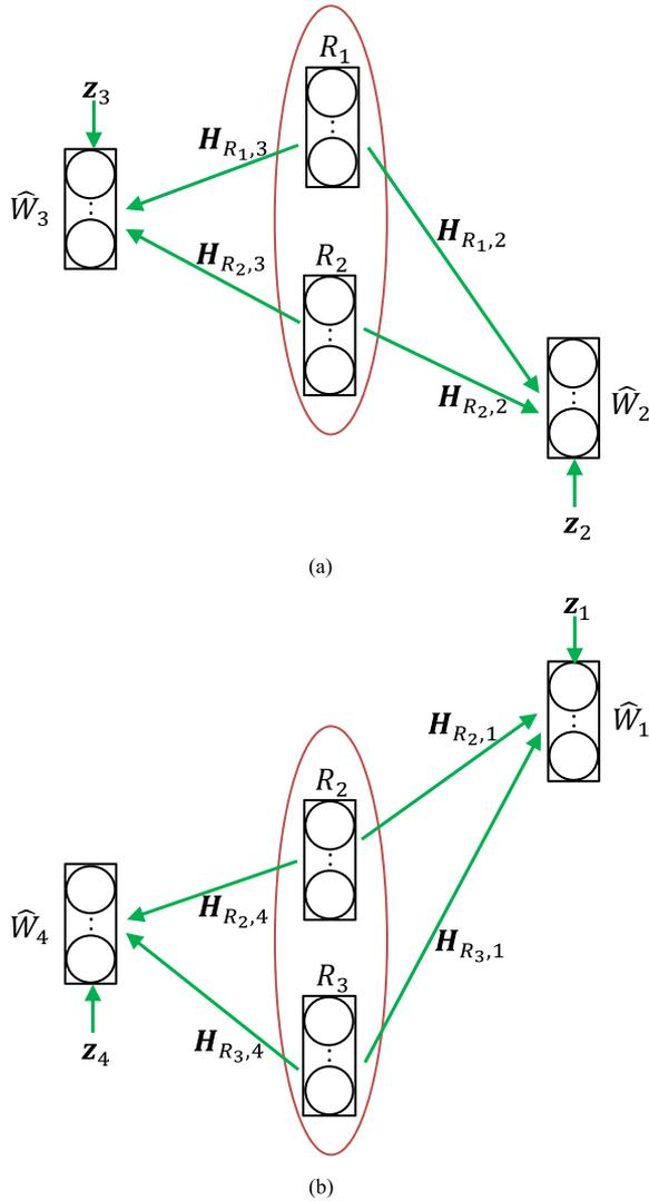
Fig. 7. The cut-set bounds from the relays to receivers in a two-way MIMO butterfly network. (a) The cut-set bound between  $R_1, R_2$  and  $D_2, D_3$ . (b) The cut-set bound between  $R_2, R_3$  and  $D_1, D_4$ .
