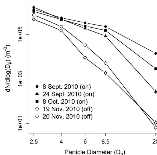
**Figure 3.** NTC coarse aerosol particle size distribution by sample date, with aerator status (on/off) noted. Vertical lines denote standard error for each point, if error bars are larger than plot point character.
