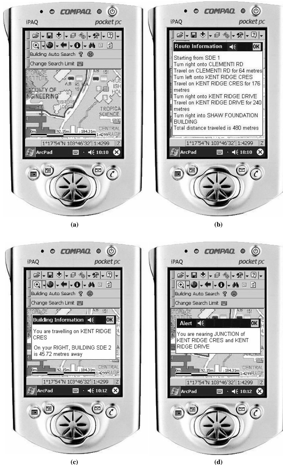
FIGURE 2 PDA visualization: (a) iPAQ with route displayed on map, (b) pretravel route instructions, (c) voice cue example, and (d) alert message.
