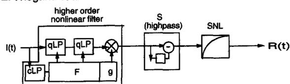
FIGURE 6. Schematics of five computational models that produce a response  $R$  as a function of time  $t$  given the input intensity  $I$  as a function of time. The models are from: (A) Sperling and Sondhi (1968); (B and C) Graham and Hood (1992); and (D) von Wiegand *et al.* (1995). See text for details.
