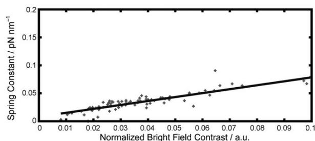
**Figure 5.** Representative scatter plot from an LD optical trap calibration experiment. Within the size range of LDs used in this experiment, the spring constant of the optical trap is quite linear in the bright field contrast of the LD image. This relationship is used to calculate the optical trap spring constant for the LDs that are trapped in the cytoplasm.
