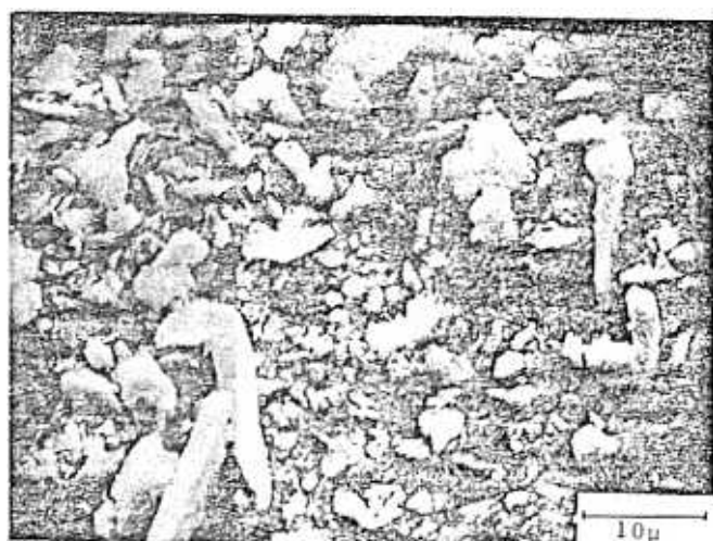
Fig. 3 Scanning electron photomicrographs and EDAX analysis of (a) (top pair) unwashed coarse hematite; (b) (centre pair) washed coarse hematite; and (c) (bottom pair) hematite slime obtained by washing
