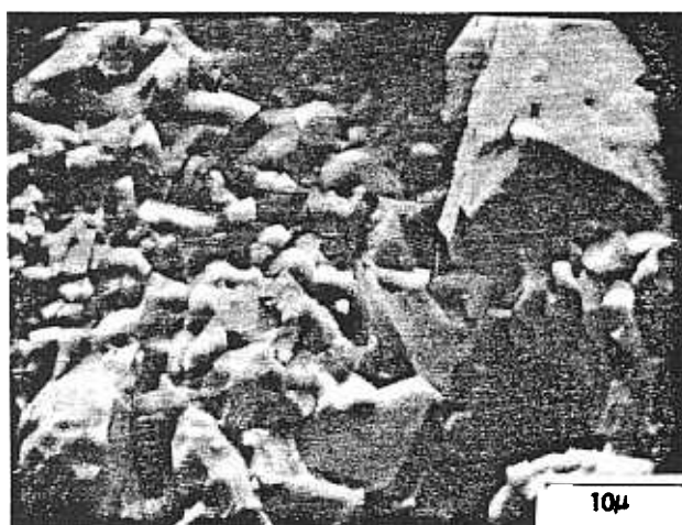
Fig. 5. Typical scanning electron micrograph of an ultrasonically treated hematite sample (No. 6).
