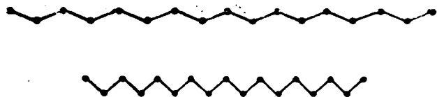
Fig. 1. Longitudinal accordion mode of an extended normal hydrocarbon molecule.
