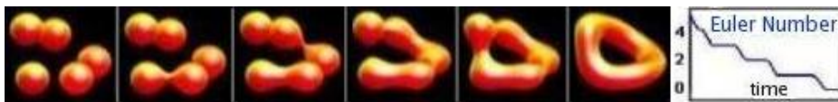
Figure 8: A phase field simulation of a few spherical like vesicles merge into a single vesicle through topological transformation, and the corresponding phase field Euler number computed on-the-fly [46].
