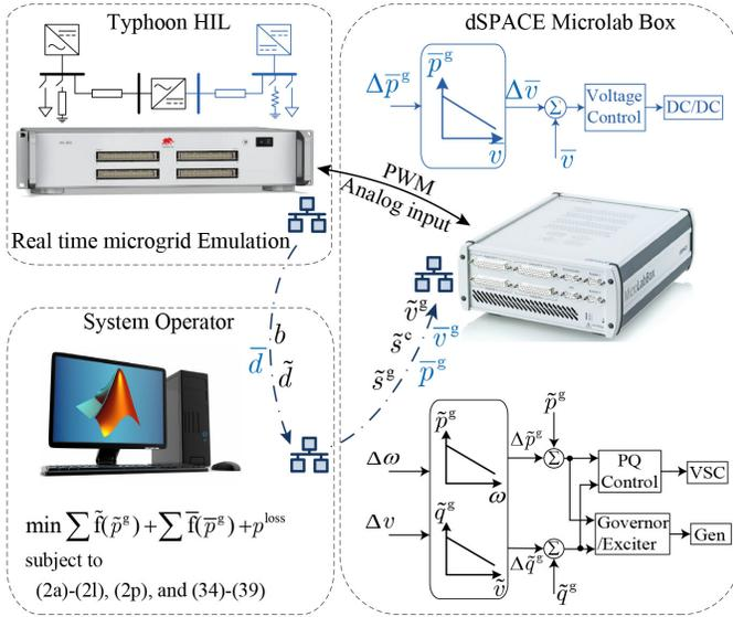
Fig. 3. HIL implementation of the AC/DC microgrid test system indicating the functionality of individual units and information flow.
