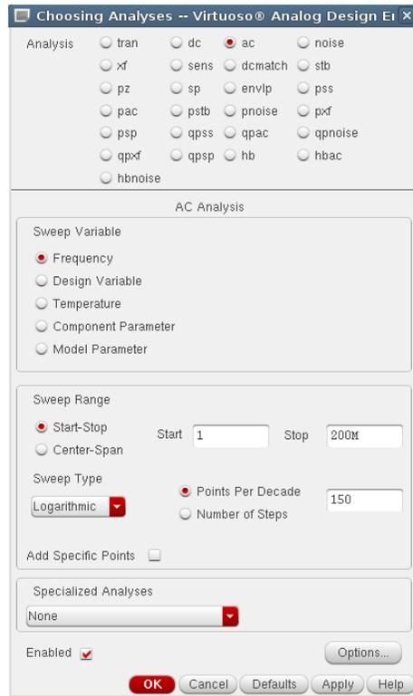
Figure 13: AC Analysis Setup
