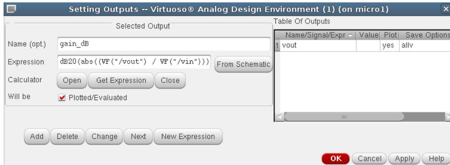
Figure 15: Set Gain Output
