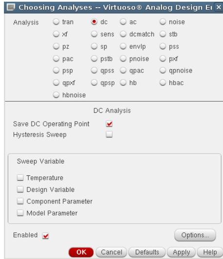
Figure 14: DC Analysis Setup
