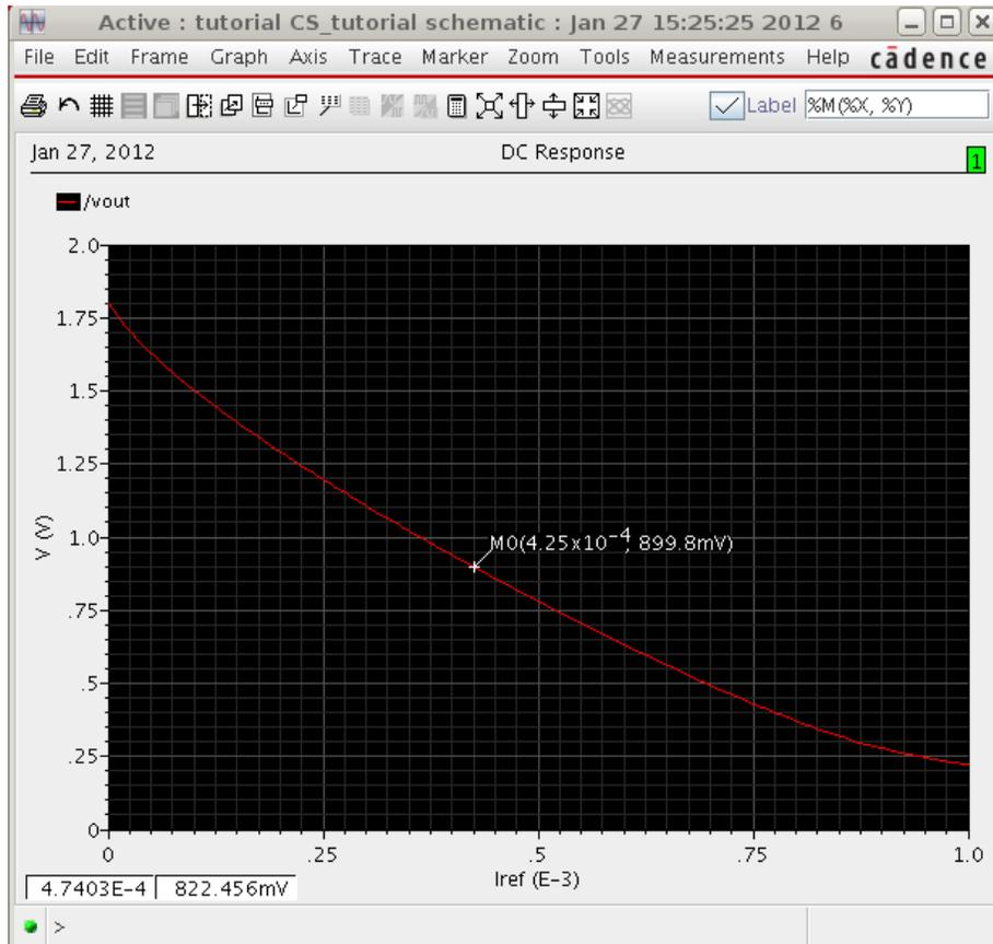
Figure 12:  $V_{out}$  (V) vs.  $I_{ref}$  (mA)
