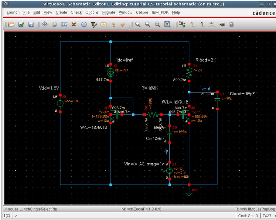
Figure 3: Schematic Window
