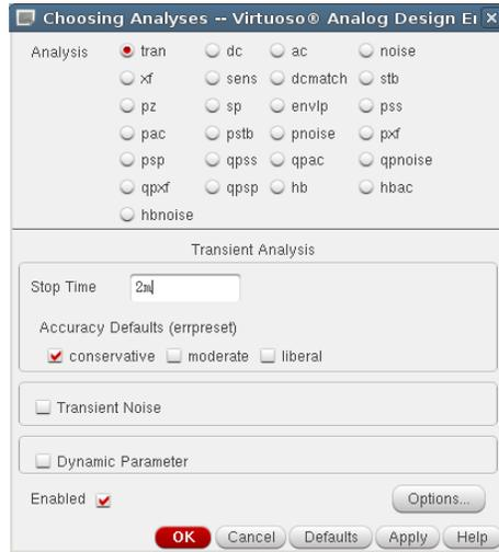
Figure 18: Transient Analysis Setup
