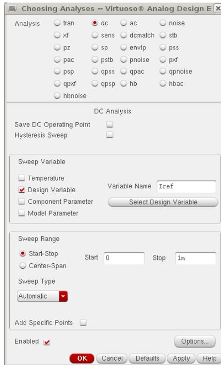
Figure 10: DC Sweep Analysis Setup
