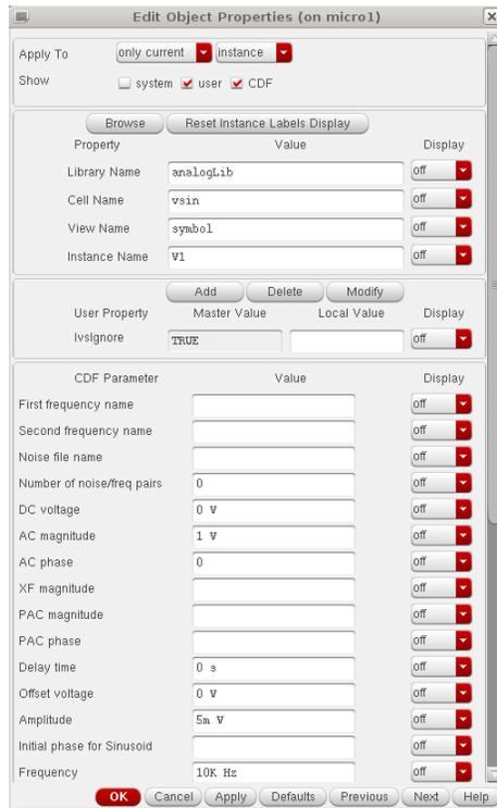
Figure 17: Edit Input Voltage Source vsin for Transient Analysis
