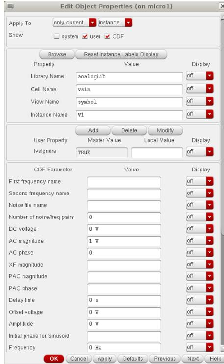
Figure 7: Edit Input Voltage Source vsin
