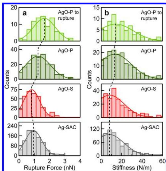
**Figure 4.** (a) Histograms of rupture force and (b) stiffness for Ag-SAC (gray), AgO-S (red), AgO-P (dark green), and AgO-P to rupture (light green). Gaussian fits are overlaid as solid curves and the dashed lines are provided as visual guides connecting the peak values.
