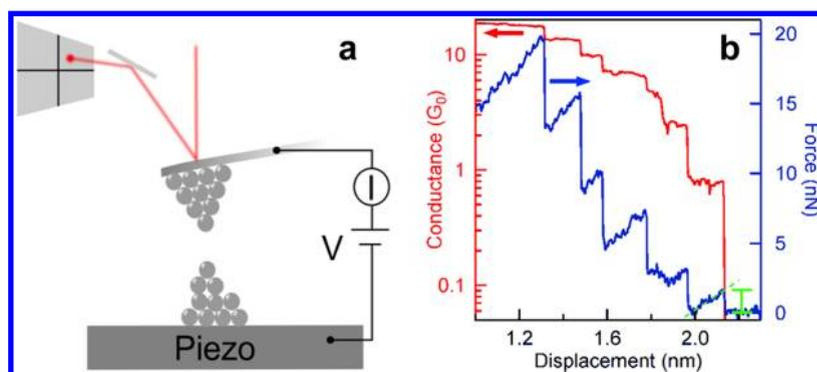
**Figure 1.** (a) Schematic of the experimental setup used for simultaneous force and conductance measurements. (b) Sample trace showing the evolution of conductance (red, left axis) and force (blue, right axis) for a Ag point contact as a function of junction elongation. The drop in force at the end of the conductance step corresponds to the rupture force, while the slope of the force trace over the conductance plateau is related to the stiffness of the junction.
