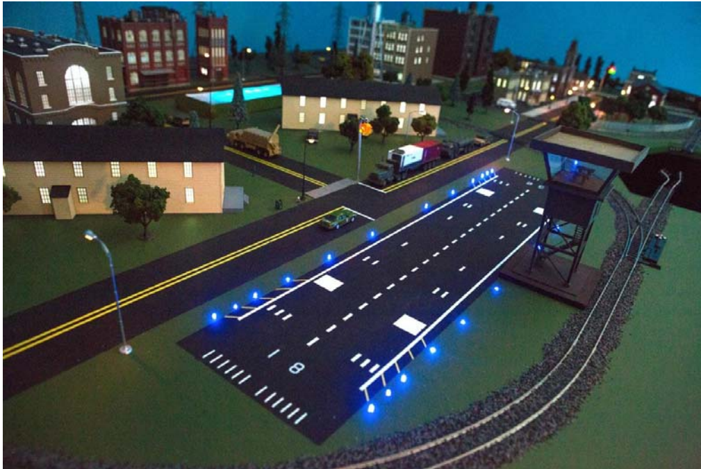
Figure 2: CyberCity is a small scale mock-up of a city, including its key underlying computing, networking, and critical infrastructure systems using real-world back-end components. 7
