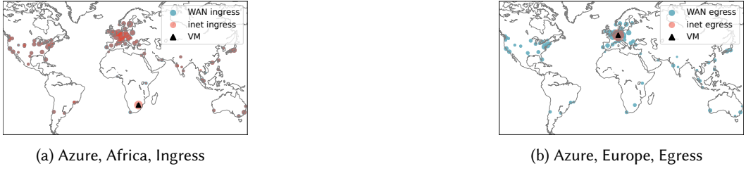
Fig. 22. Geographical distributions of the ingress/egress cloud edges for RIPE Atlas probes to reach different network service tiers of the Africa and Europe regions for Azure. The legend definition is the same as Fig. 21. This figure shows the results of the first measurement (Table 5).
