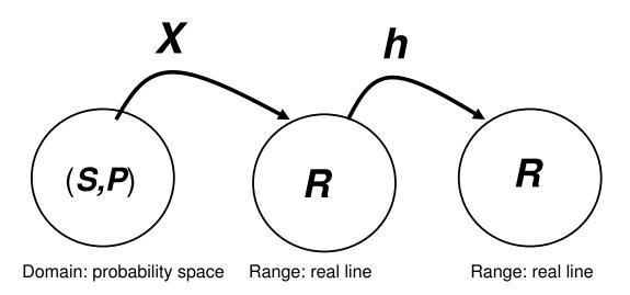
Figure 2: A (real-valued) function of a random variable is itself a random variable, i.e., a function mapping a probability space into the real line.
