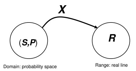
Figure 1: A (real-valued) random variable is a function mapping a probability space into the real line.
