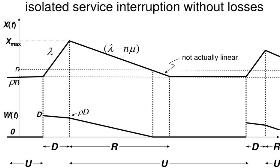
**Figure 1** Sample paths of the approximating number in system,  $X(t)$ , and the associated waiting-time process,  $W(t)$ , in the pure-delay system experiencing an isolated exogenous service interruption.
