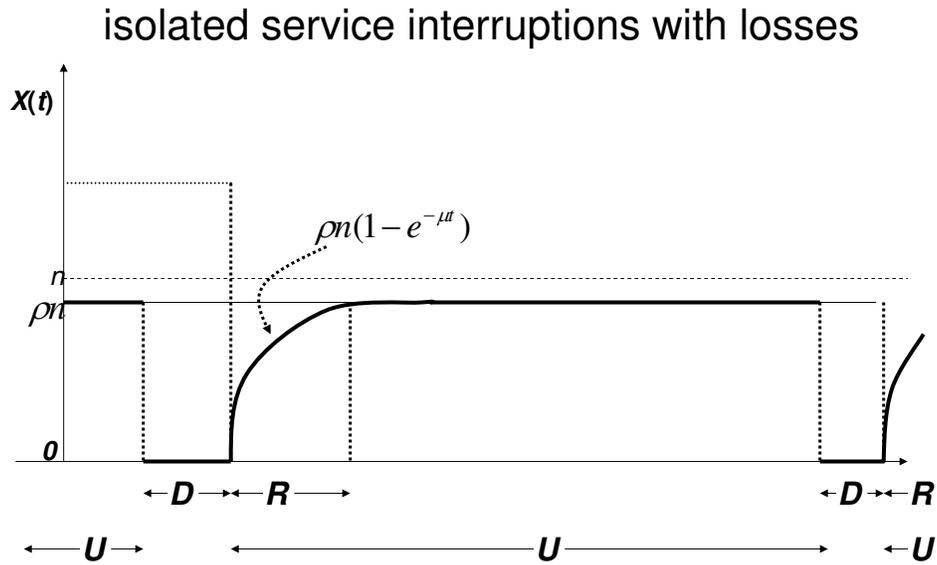
**Figure 2** The number in system,  $X(t)$ , in the pure-loss fluid model with alternating up and down times distributed as  $U$  and  $D$ .
