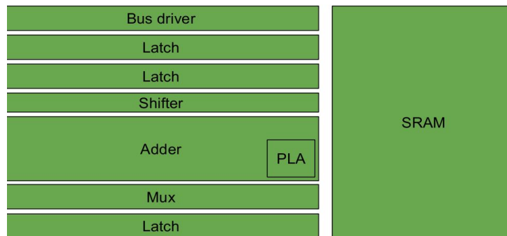
Figure 3.2 Floor Plan of Layout
