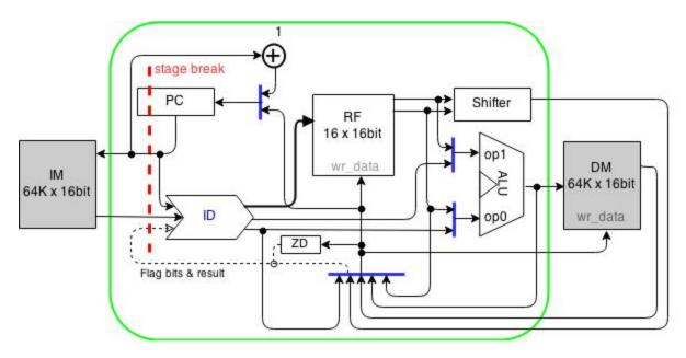
By the end of this course, you will build a complete simplified 16-bit ARM based CPU. The 2-stage pipelined CPU will breakdown the stages between the instruction fetch and instruction decode as shown with the red dotted line in the diagram.
