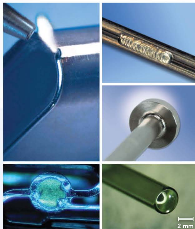
FIGURE 2. Typical processing results on typical medical devices: pacemaker (top left), welded wire stent (top right), endoscope flange weld (center right), stent marker weld (bottom left), and sealing of glass tracers (bottom right).
