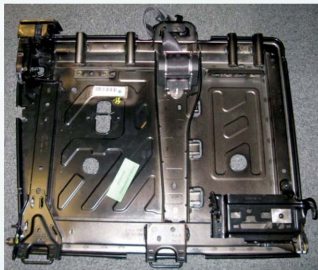
FIGURE 4. Rear seat structure with weld close up.
