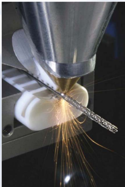
FIGURE 4. Laser cutting of stents using ROFIN workstation StarCutTube.
