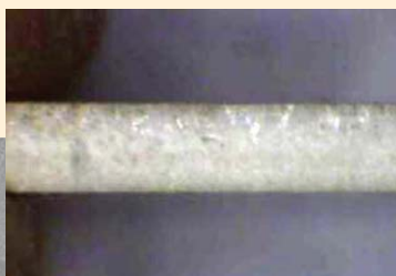
FIGURE 2. (top) 1.2 mm alumina ceramic (96%), 250 mm/min, air assist gas; (bottom) 0.5 mm alumina ceramic (99.7%), 650 mm/min, air assist.
