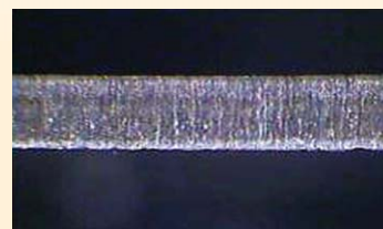
FIGURE 1. (top) 1 mm alumina ceramic (96%), 300 mm/min, air assist gas; (bottom) Trepanned hole (0.5 mm dia.), 0.6 mm alumina ceramic (99.7%), 200 mm/min, air assist gas.
