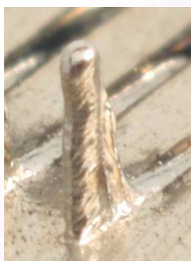
FIGURE 3. Left: SEM image of a series of linear surface features in titanium. Right: Photo of the same feature. Note the level of reproducibility in the features.
