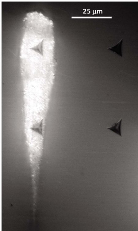
Fig. 16 Reflection DIC optical microscopy of 2 \mu\text{m} depth nanoindentations on and off the femtosecond laser-irradiated region for fracture toughness measurements
