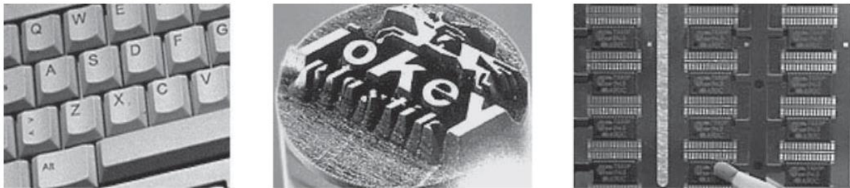
Figure 6: Laser marking examples. (Left) A PC keyboard; (Middle) graphite electrode for EDM; and (Right) Laser marking of electronic components. (Courtesy of ALLTEC GmbH Inc.)
