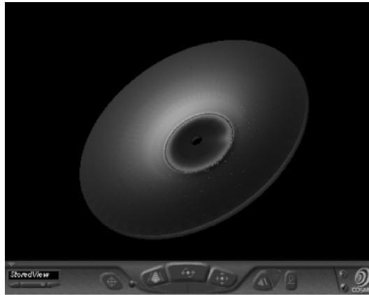
Figure 7. Snapshot of a 3D interactive animation of temperature history in laser forming of a circular plate.
