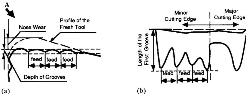
Fig. 1. Groove wear at the minor cutting edge: (a) view from tool top face; (b) view from A.
