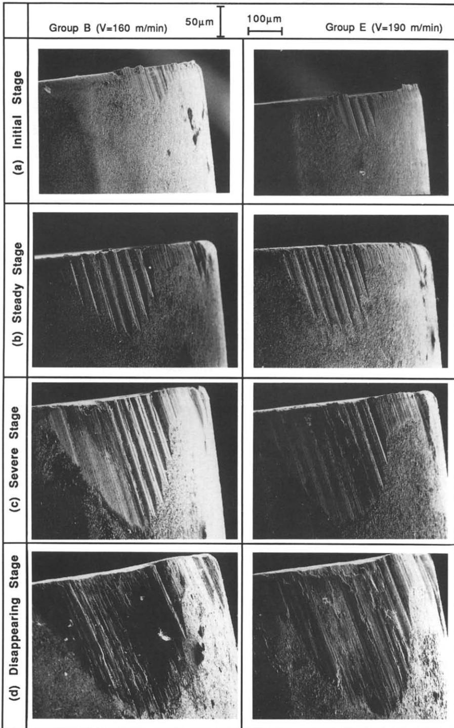
Fig. 8. Groove wear development under the lower feed condition ( $0.04$  mm rev $^{-1}$ ).
