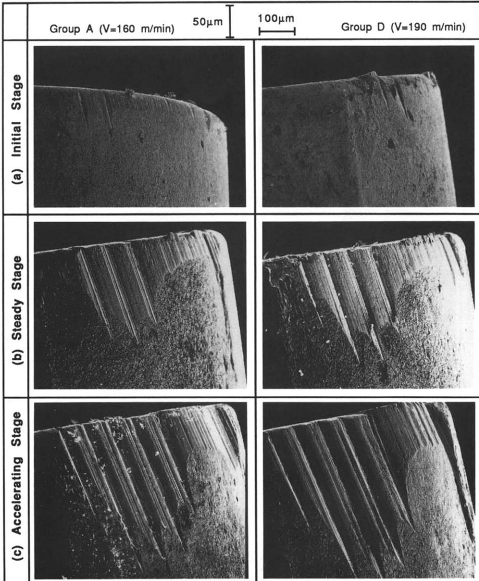
Fig. 9. Groove wear development under the higher feed condition ( $0.08 \text{ mm rev}^{-1}$ ).
