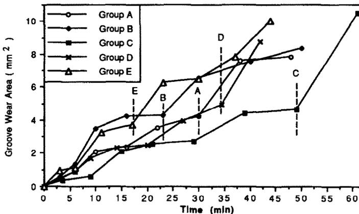
Fig. 5. Development of groove wear area.
