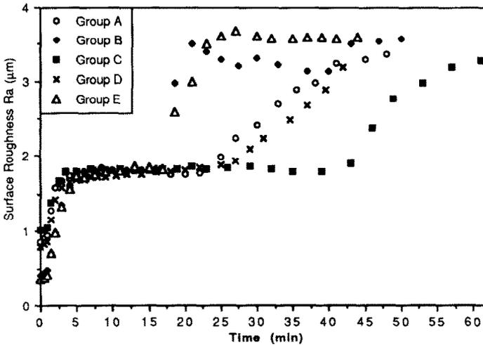
Fig. 7. Surface roughness for five cutting conditions.
