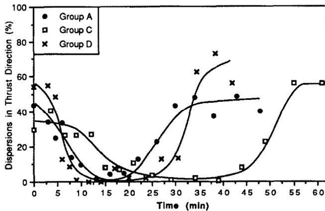
Fig. 11. Dispersion patterns for the higher feed condition ( $0.08 \text{ mm rev}^{-1}$ ).
