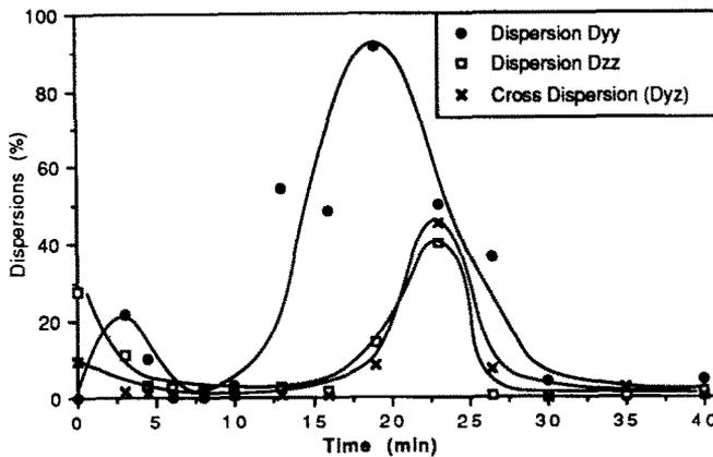
Fig. 10. Dispersion patterns for the lower feed condition ( $0.04 \text{ mm rev}^{-1}$ ).
