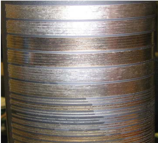
Fig. 6 Coated laser tube forming using circular beam
