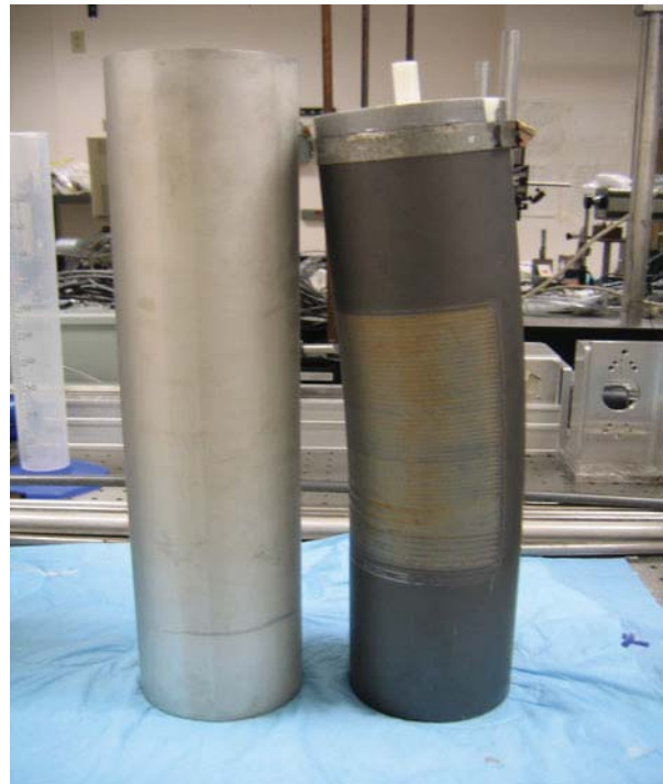
Fig. 10 The first SS321 tube bent with the rectangular beam, graphite coating, plug, and fast active cooling
