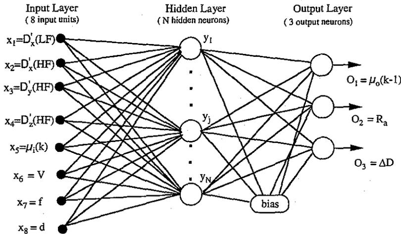
FIG. 3 THE STRUCTURE OF A 3-LAYER BP NEURAL NETWORK
