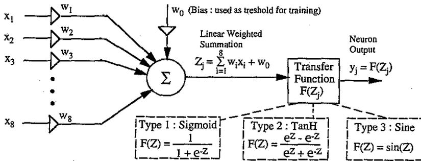
FIG. 4 ALGORITHM OF A PERCEPTRON NEURON IN BP NEURAL NETWORK
