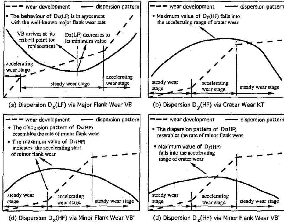
FIG. 2 FOUR DISPERSION PATTERNS RELEVANT TO THE PROGRESSIVE TOOL WEAR
