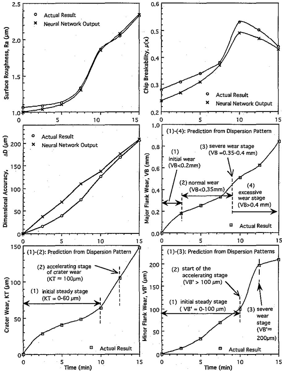
FIG. 6 A REPRESENTATIVE EXAMPLE OF THE TESTING RESULTS OF THE OVERALL MACHINING PERFORMANCE FOR A SOFT FLAT-FACED TOOL ( $V = 140\text{m/min}$ ,  $f = 0.12\text{mm/rev}$ ,  $d = 0.5\text{mm}$ , Tool Grade = SECO 883)
