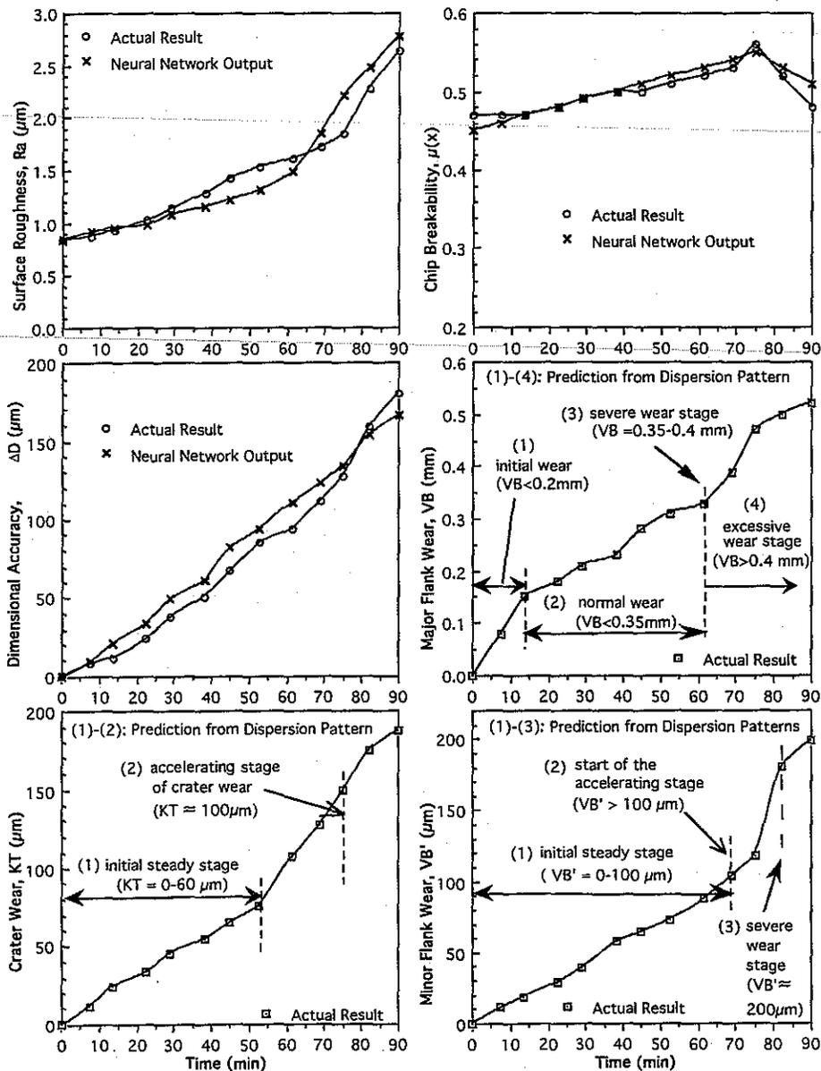
FIG. 7 A REPRESENTATIVE EXAMPLE OF THE TESTING RESULTS OF THE OVERALL MACHINING PERFORMANCE FOR A HARD GROOVE-STYLE TOOL ( $V = 170\text{m/min}$ ,  $f = 0.10\text{mm/rev}$ ,  $d = 0.5\text{mm}$ , Tool Grade = ISO P10)
