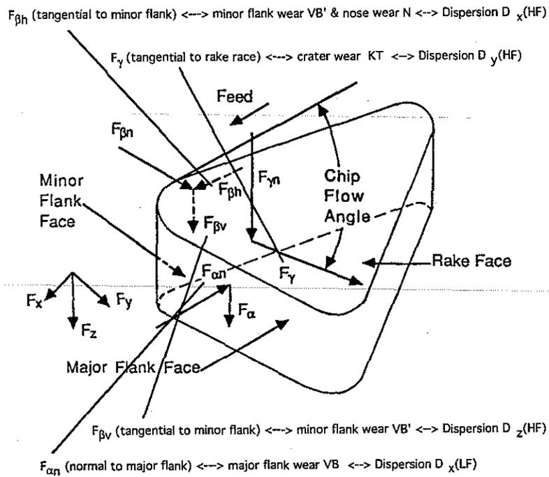
FIG. 1 INTERRELATIONSHIP BETWEEN VARIOUS TYPES OF FORCES/WEAR AT DIFFERENT TOOL FACES AND THE FOUR DISPERSION PATTERNS RECOGNISED FROM 3-D CUTTING FORCE
