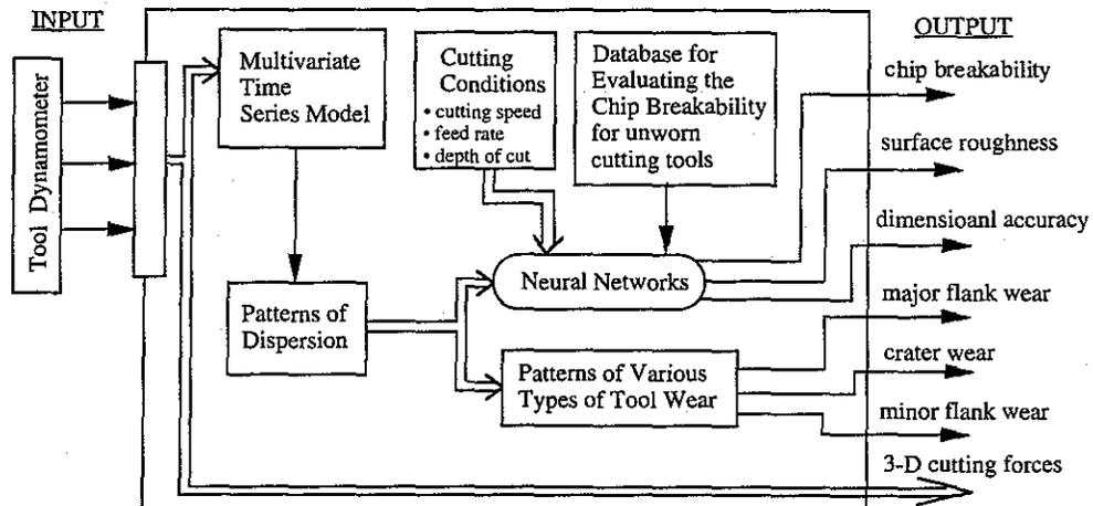
**FIG. 5** A SINGLE SENSOR BASED MULTI-FUNCTIONAL MONITORING SYSTEM FOR IN-PROCESS EVALUATING THE OVERALL MACHINING PERFORMANCE
