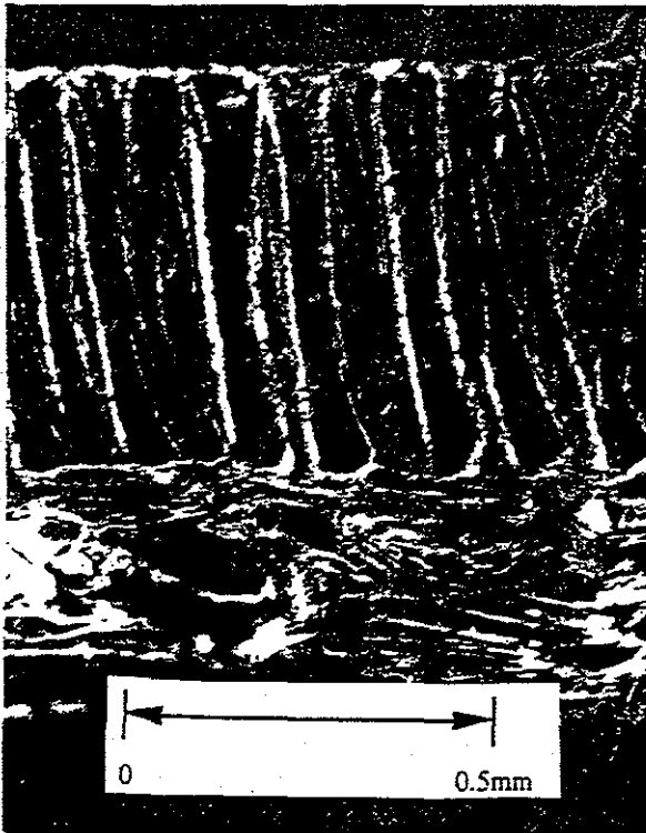
Figure 3. The periodic striation pattern observed in specimen 7
