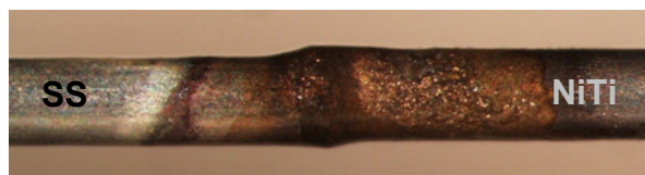
Figure 3: Optical micrograph of dissimilar metal joint between NiTi and Stainless Steel. Irradiated on SS.
