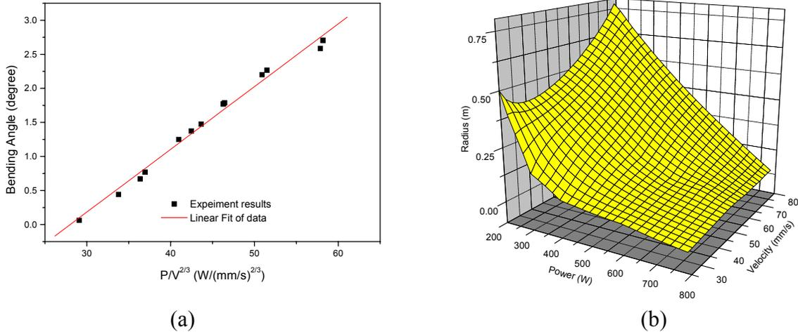
Figure 2. (a) Bending angle and (b) radius of curvature vs. power/velocity, based on experimental data of 1010 steel coupons of 80 by 80 by 0.89 mm with laser beam size of 4 mm.
