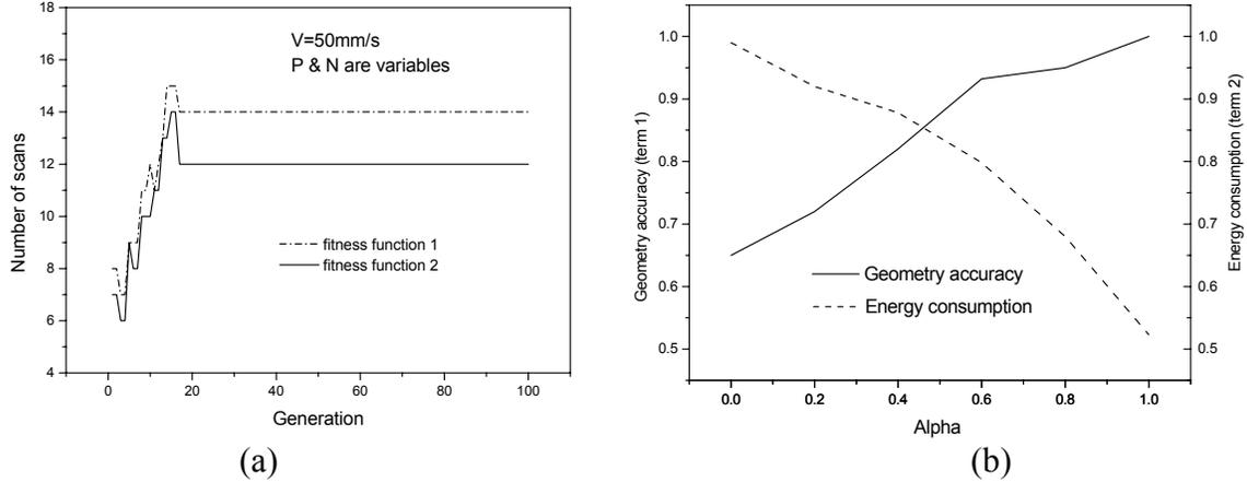
Figure 5. (a) Comparisons of two fitness functions; and (b) effect of weighting coefficient  $\alpha$  in Eq. 10 on the balance of competing objectives.
