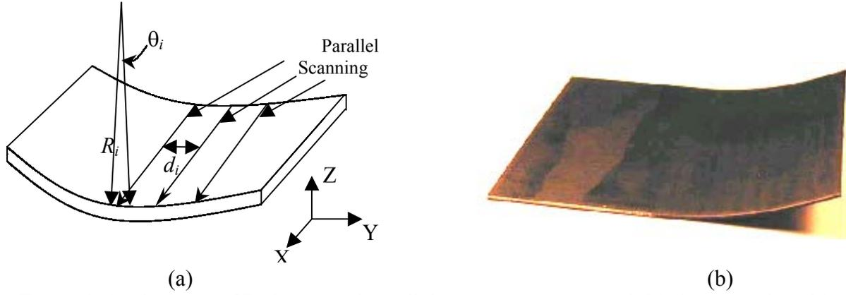
Figure 1. (a) A class of 2D shapes and parallel scanning pattern; and (b) sheet metal (mild steel) after being laser formed using the scanning pattern in (a).
