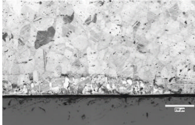
Figure 2: Optical micrograph of 718 recrystallization caused by high-temperature laser forming
