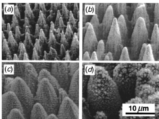
Fig. 5. SEM images of the conical silicon microstructures formed by femtosecond laser irradiation in a background gas of (a) SF<sub>6</sub>, (b) Cl<sub>2</sub>, (c) N<sub>2</sub>, and (d) air [29].
