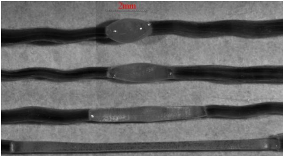
Figure 8: Joint morphologies obtained from various degrees of fiber constraint and tension. Joint length and fiber packing are both affected by bundle tension.
