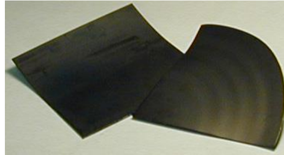
FIG. 2 TYPICAL LASER FORMED SAMPLES USING THE SCANNING SCHEMES SHOWN IN FIG. 1.
