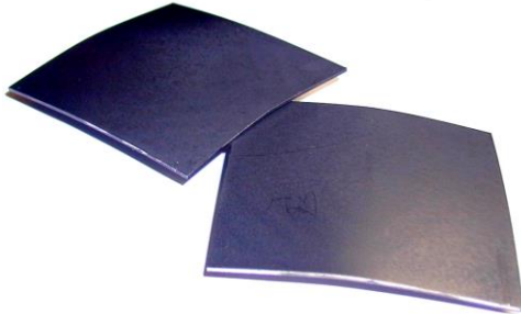
FIG. 9 LASER FORMED AISI1010 STEEL PLATES USING THE SCANNING PATHS AND HEATING CONDITIONS INDICATED IN FIG. 8.
