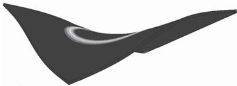
FIGURE 9. DISTORTIONS INDUCED BY CIRCULAR PATH WELDING
