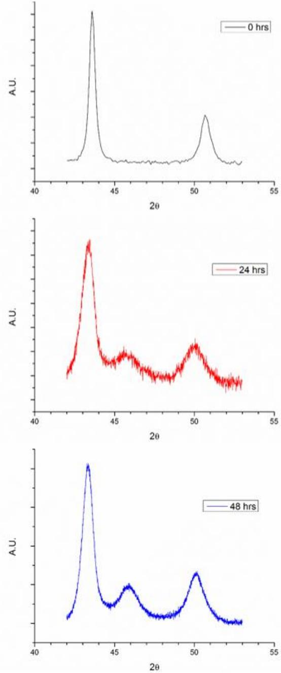
Figure 2 XRD measurements of lattice changes from cathodic charging a specimen without LSP treatment.
