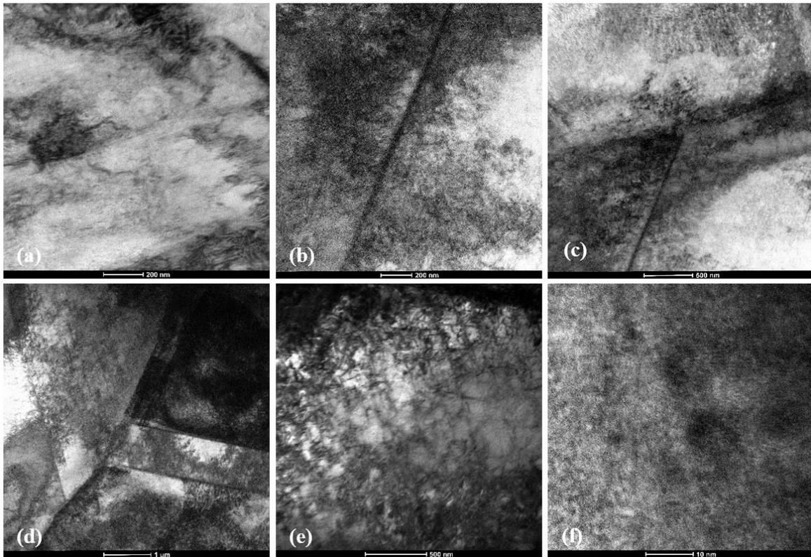
Figure 8 TEM images of untreated AISI 304 stainless steel (a), after 3 LSP impacts at  $2.25 \text{ GW/cm}^2$  (b-f). Significant increased to the dislocation density are seen in (b), and these dislocations get tangled at grain boundaries (c). The individual grains in (d) have differing dislocation behaviour. Cell formation is present in (e), and the high magnification of (f) shows the orientation of the lattice.
