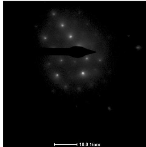
Figure 9 TEM diffraction pattern in an area showing dislocation cell structure, indicating that there is not lattice misalignment across the boundaries.
