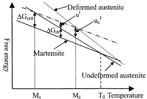
Figure 1 Free energy diagram showing the suitable conditions for the formation of deformation induced martensite [20].
