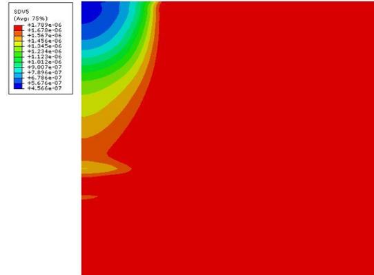
Figure 6 Distribution of dislocation cell size after 3 LSP impacts. Symmetry is used along the boundary at the left side.
