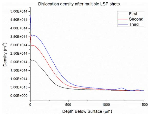
Figure 5 Increases to the dislocation density after LSP processing, which act as an impediment to hydrogen induced martensite formation. The largest increase is seen upon the initial incident pulse.
