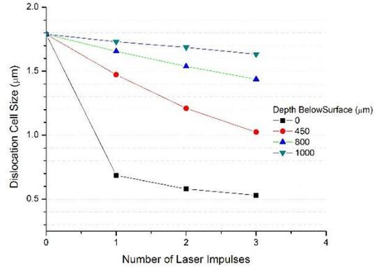
Figure 7 Dislocation cell size for increasing number of incident LSP pulses at 4 depths.
