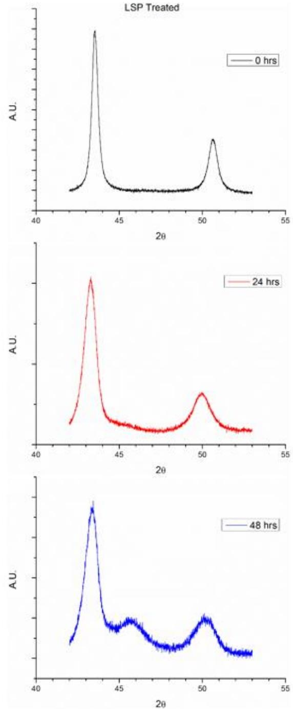
Figure 4 XRD measurements of a selected region of the spectrum for samples after LSP processing (a), and then subjected to 24 hours (b) and 48 hours (c) of cathodic charging. The initially austenitic peaks experience broadening after 24 hours, but no martensite formation occurs, illustrating the effectiveness of LSP processing as a mitigation tool. Some martensite does eventually form after 48 hours.
