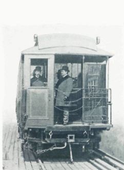
DETAILS OF PLATFORM, CAB AND MASTER CONTROLLING MECHANISM—SPRAGUE MULTIPLE UNIT TRAIN—1898
