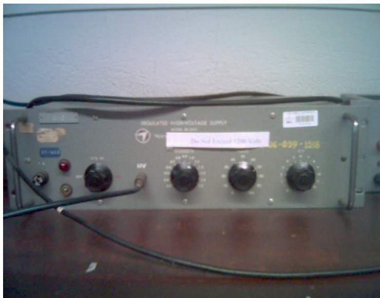
Figure 2: The High Voltage Power Supply, which supplies voltage to the detector tube. The power switch and indicators are at left; the voltage is controlled by the three knobs at center and right.
