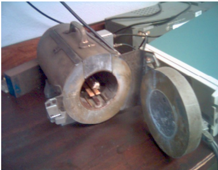
Figure 1: The Geiger counter. The actual detector is the tube at center; sources are placed on the small wooden trays below the detector.
